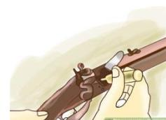
6. Bring the gun up into the aim & bring the hammer into the full cock position. The gun is now ready to fire.
